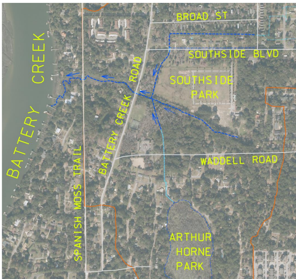
Figure 2.1 –Basin #2 ditches and Battery Creek outfall
