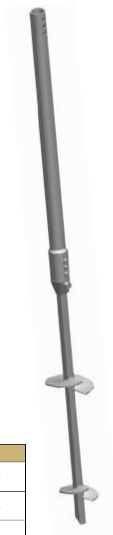
Pile Assembly with Transition Coupler Figure 7-38
