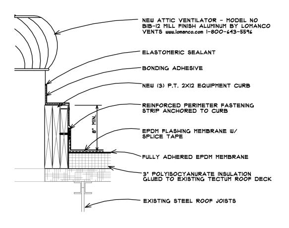
A5 NEW TURBINE VENT FLASHING
