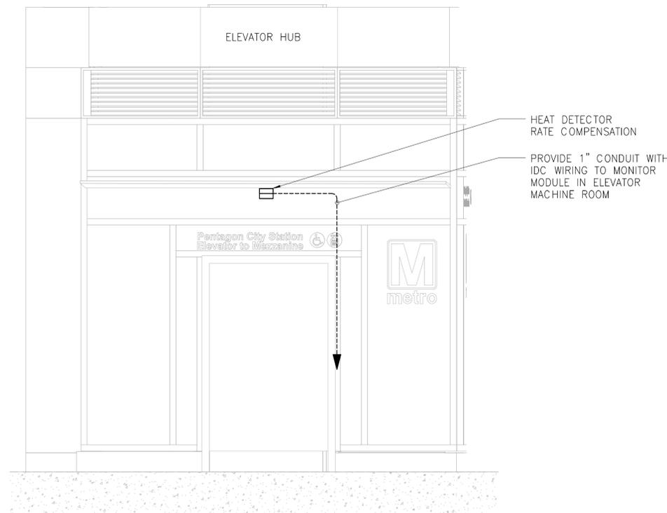
**4** STREET LEVEL - SOUTH ELEVATION - FIRE ALARM DEVICES
