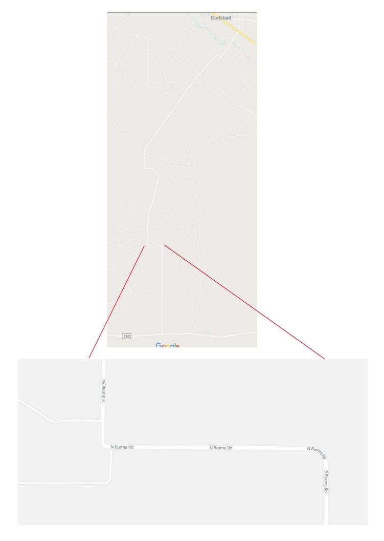
Taper approximately 20' from 4" to nominal overlay for transition from overlay to current paving. Taper shall not enter into low water crossing. Taper approximately 150' from 4" Taper approximately 150' from 4" to to nominal overlay for transition nominal overlay for transition from overlay from overlay to current paving. to current paving. 65' 150' Carlshad Loop
