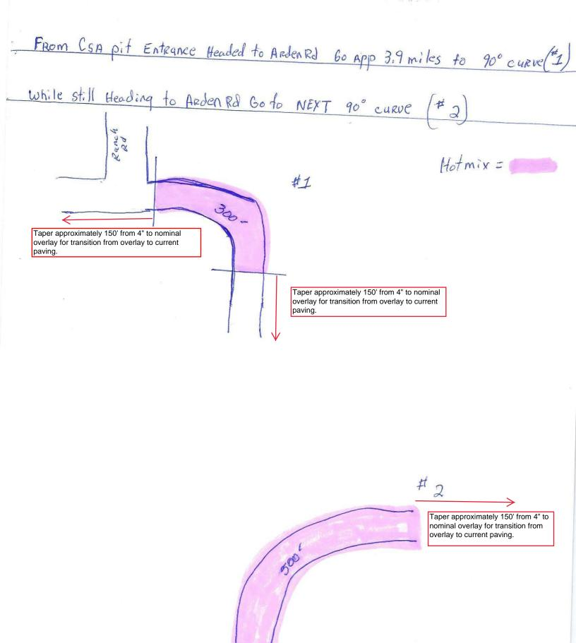
Taper approximately 150' from 4" to nominal overlay for transition from overlay to current paving.
