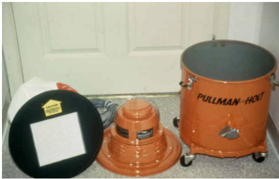
FIGURE 8.5 One example of a commercial-type HEPA vacuum.
