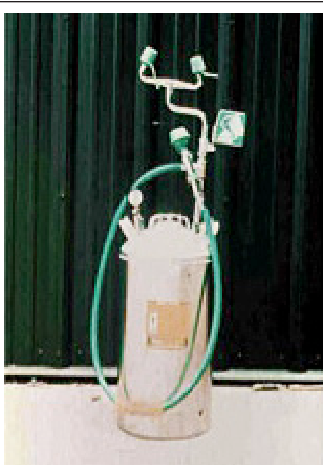
FIGURE 12.21 Eye- and body-wash stations are required when working with corrosive or irritant chemicals.
