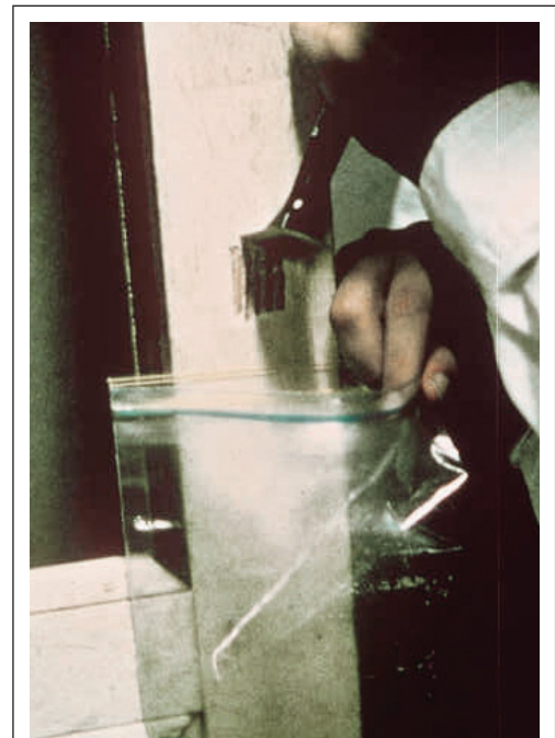
FIGURE 7.5 Removing paint-chip sample.
