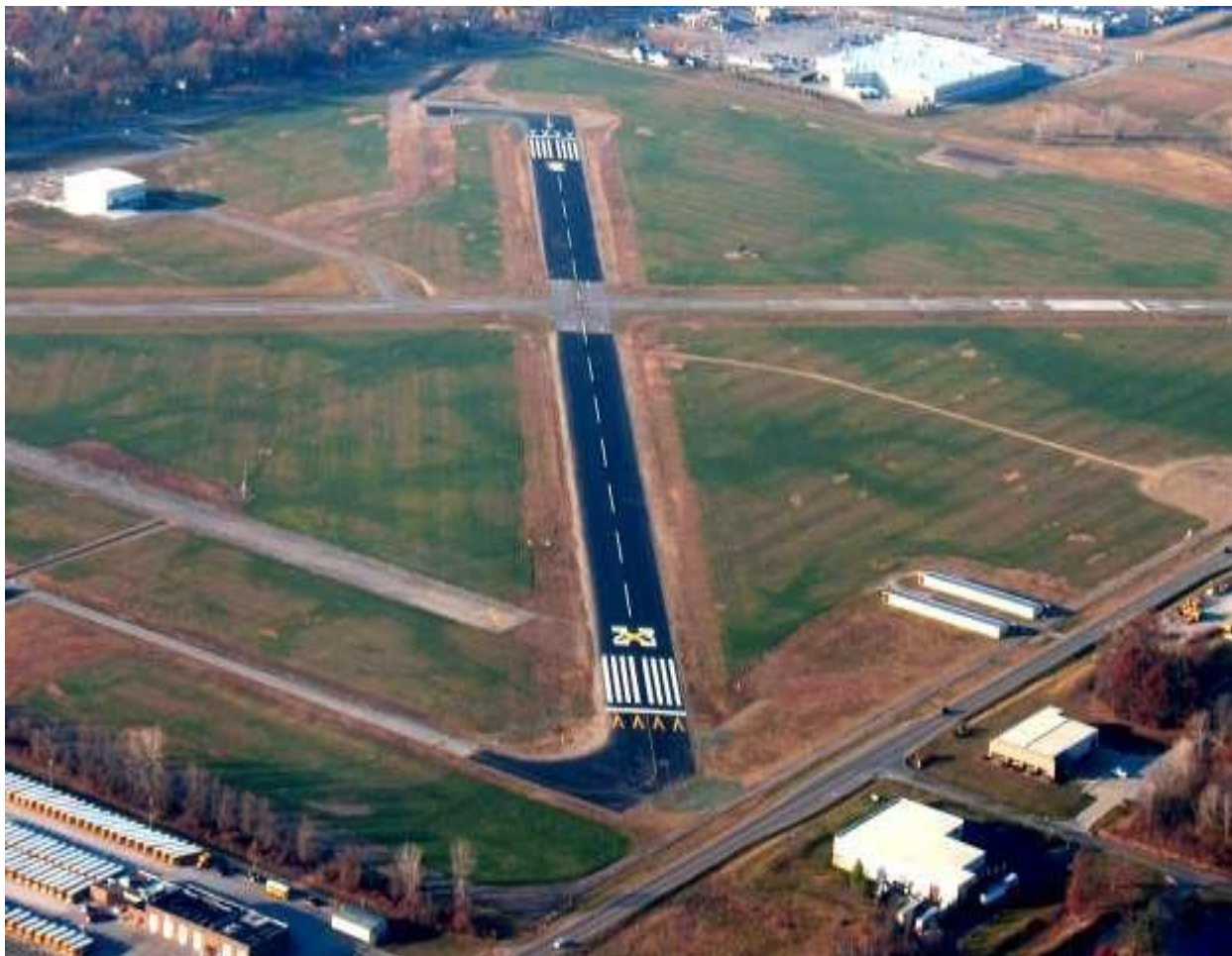
Figure 2-1 Markings for a Temporarily Closed Runway
