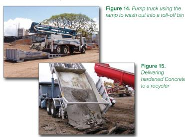
Figure 15. Delivering hardened Concrete
