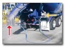
Figure 8. Chute washout bucket and pump
