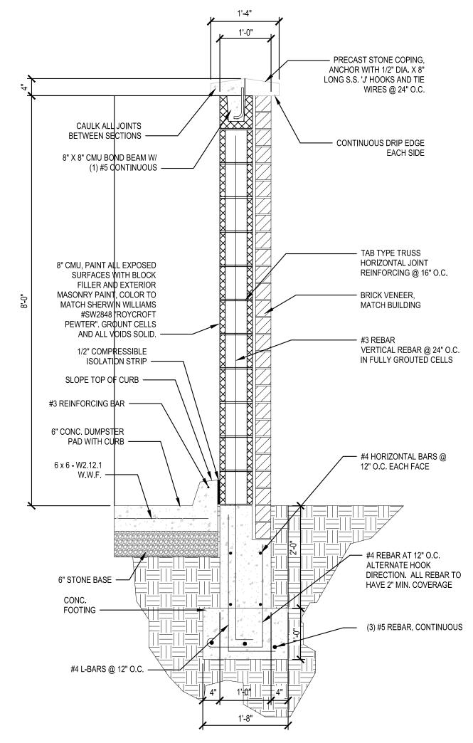
4 Dumpster Enclosure Wall Section
