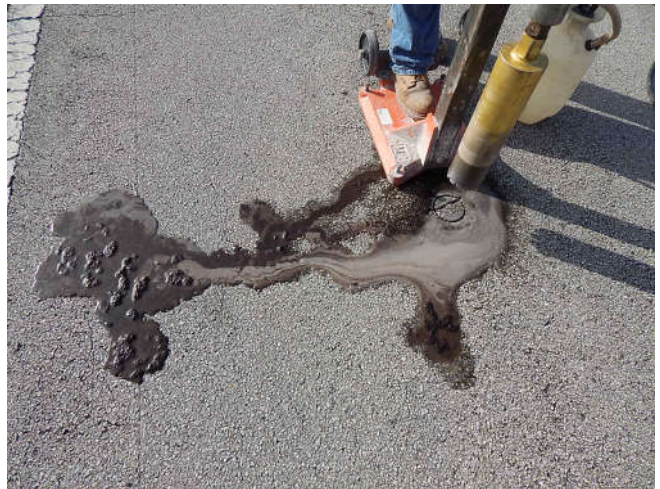
Photo 10: Weak asphalt matrix washing out of core hole C-4
