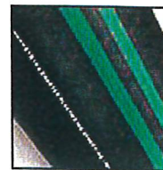
C906 HDPE (Green stripes [force main sewer])
