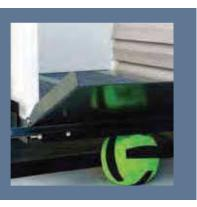
Automatic folding ramp provides easy entry when lift is lowered and additional stability when lift is raised
