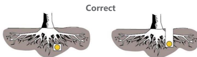
Figure 1: Tunnel to minimize root damage (left) as opposed to surface-dug trenches in root zone (right)
