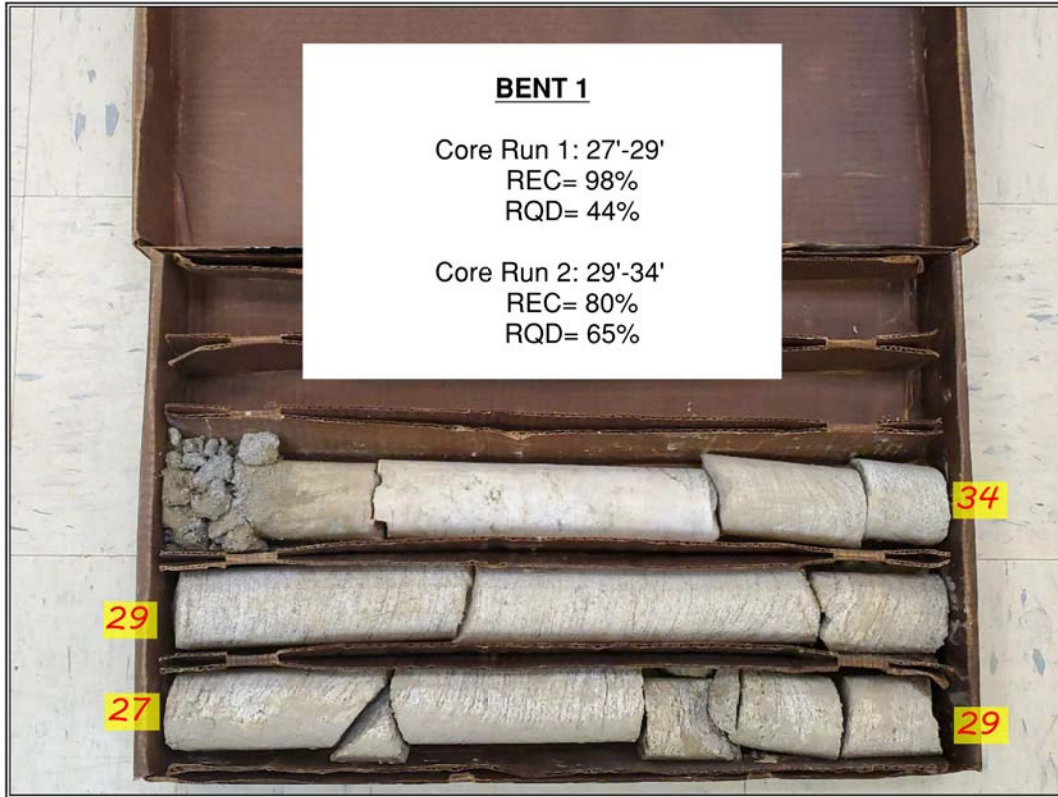
Rock Core from Boring Bent 1 (27' – 34')
