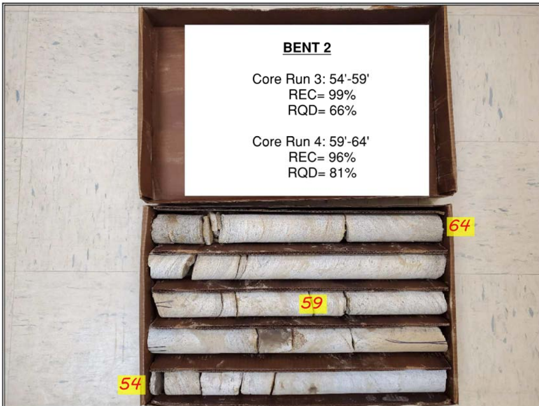
Rock Core from Boring Bent 2 (54' – 64')
