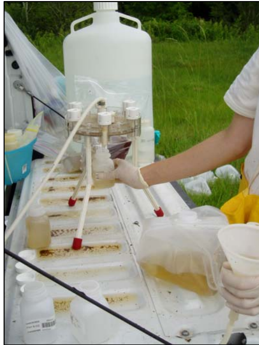
Photograph 19. Geotech pump and P Meter.
