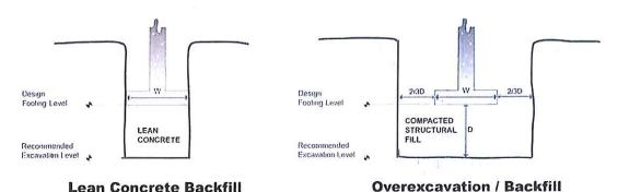
NOTE: Excavations in sketches shown vertical for convenience. Excavations should be sloped as necessary for safety
