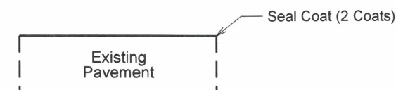
Loraine Street Seal Coat Section
