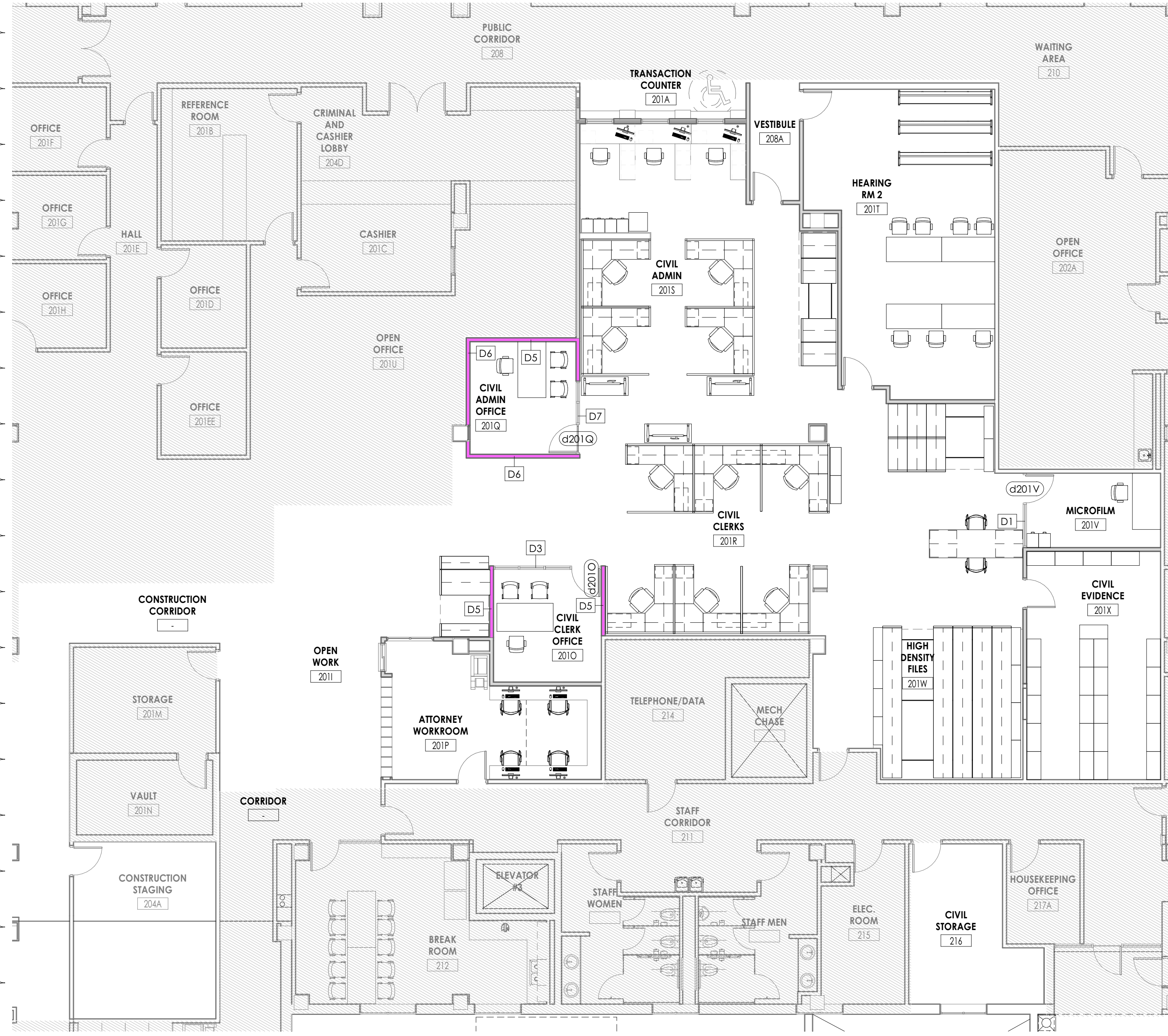
LVL 02 - FURNITURE/DEMOUNTABLE PARTITION PLAN - PHASE 2 1/8" = 1'-0" REFER TO A101 SERIES FOR CONVENTIONAL DRYWALL PARTITIONS
