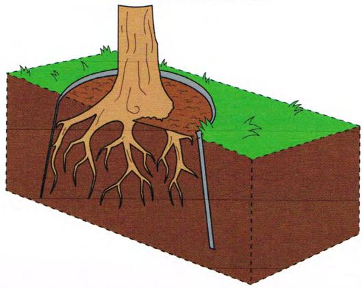
The purpose of Sidewalk Shield is to direct the root growth downward instead of out along the surface where they can do harm to sidewalks, driveways, septic systems, etc. The material is position in a 10-degree downward slope. The top (portion closer to the soil surface) should be closer to the tree than the bottom. This creates a funnel to direct roots in a downward growth pattern.
