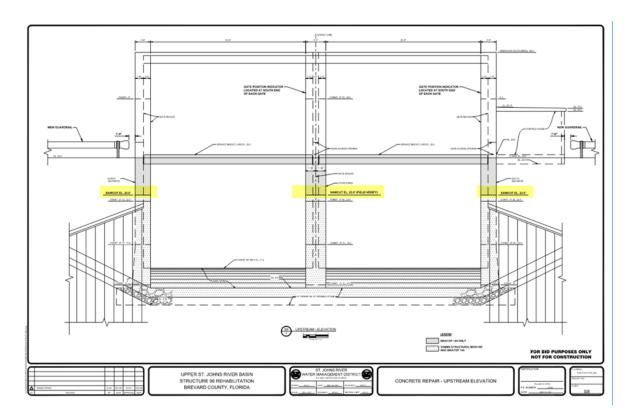
Q13: Reference S9, the construction joint at elevation 15.0. Is the intent for the south and north abutments and the center pier to be sawcut at elevation 15.0 and what is the depth of sawcut?
