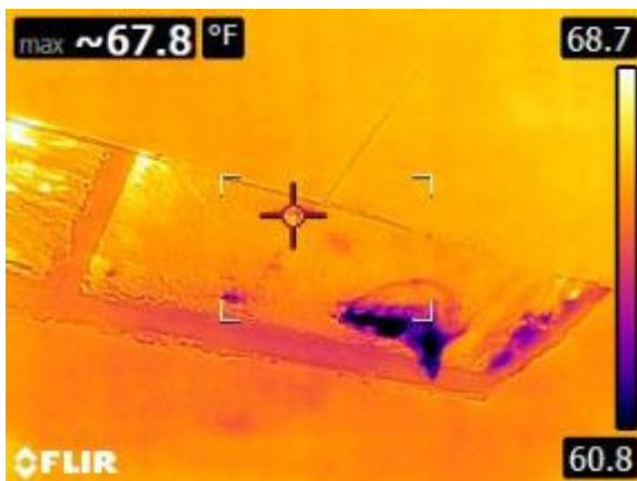
The drywall is being replaced due to condensation. The ductwork also has microbial growth.
