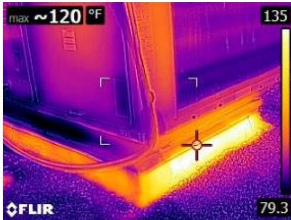
The roof curb temperature is about 120°F.
