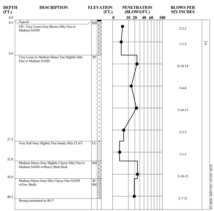
Caved at 5'. Groundwater at 5.5' at time of boring.
