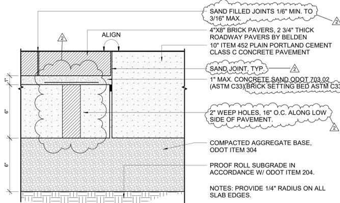
4 CONCRETE CROSSWALK PAVEMENT - (COC STD. DWG. NO. 41)
