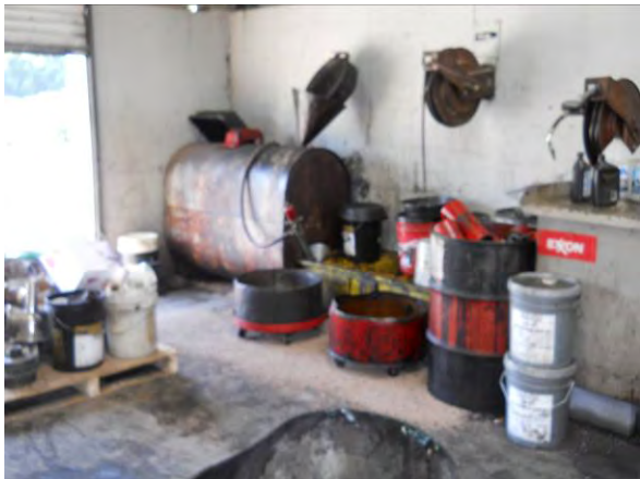
Photo #3 View of the used oil AST and various drums located inside of the garage at 159 Hamm Road.
