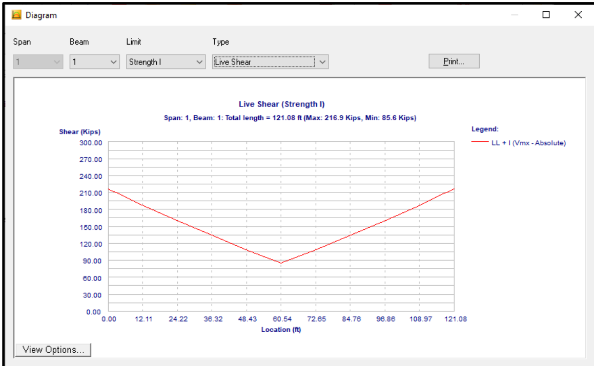
Figure 14: Strength 1 Live Load Shear, Concrete Spans
