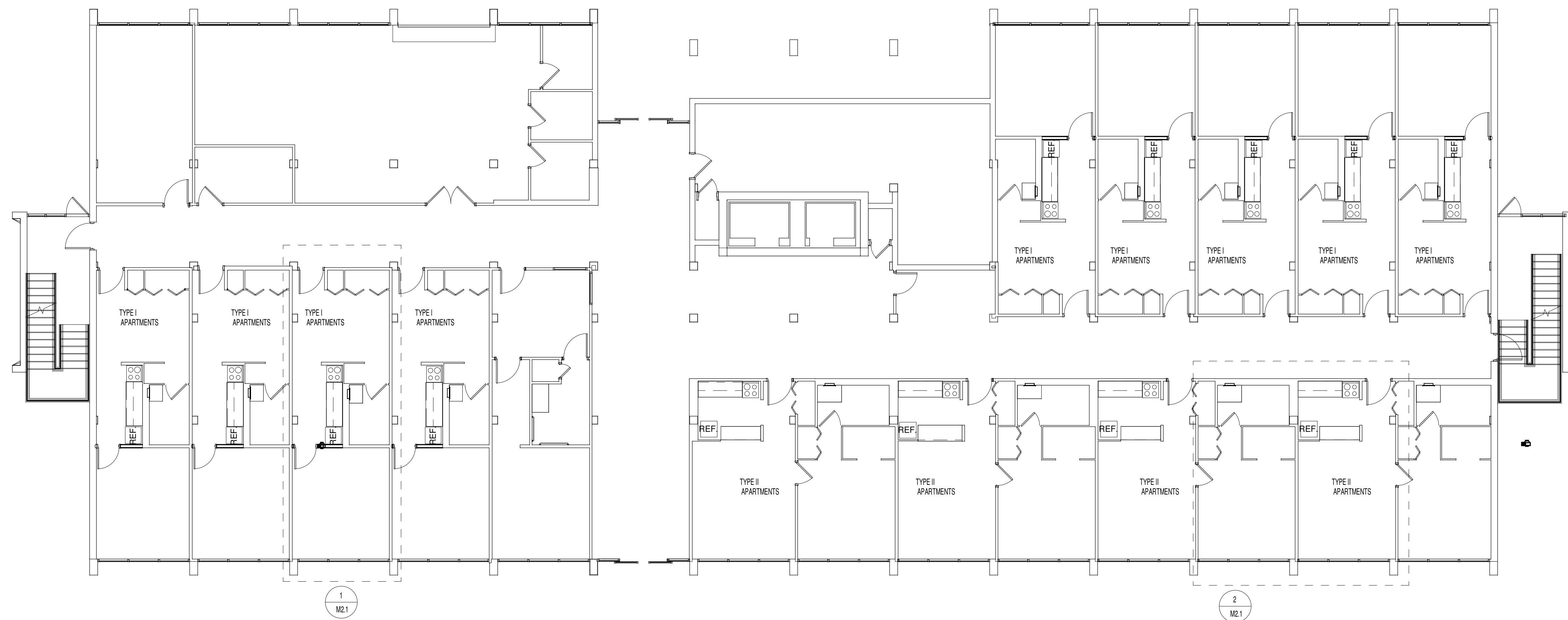
1 1st FLOOR BUILDING A HVAC 1/8" = 1'-0" GENERAL NOTE: REPLACE ALL EXISTING EXHAUST GRILLES IN RESTROOM CEILINGS WITH NEW EQUAL TO PRICE MODEL 80.12x12.
