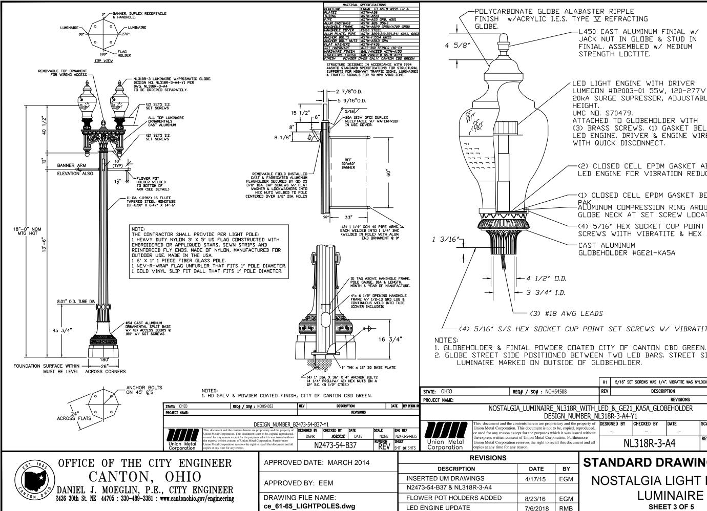
L450 CAST ALUMINUM FINIAL w/ JACK NUT IN GLOBE & STUD IN FINIAL. ASSEMBLED w/ MEDIUM STRENGTH LOCTITE.
