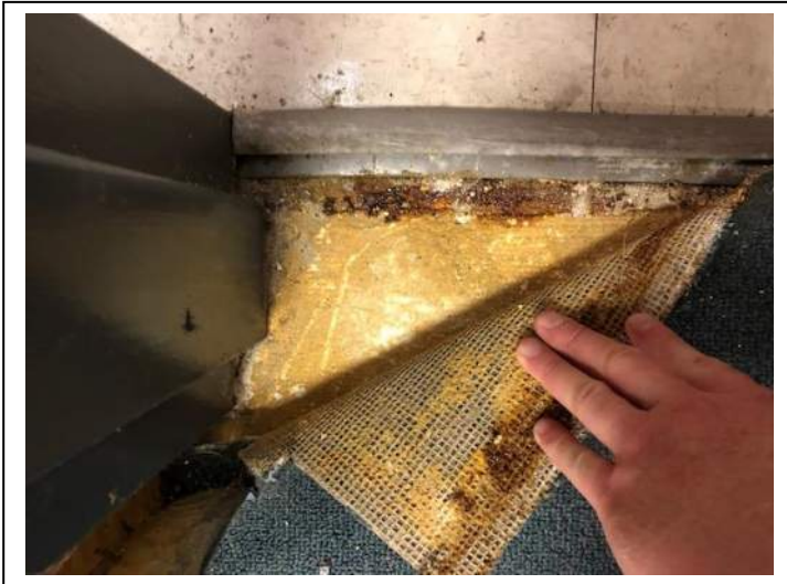
Photo #73 Material: Yellow Carpet Mastic Sample loc Sample Result: No Asbestos Detected
