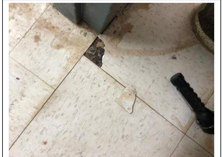
Photo #10 Material: 12"X12" White With Black Streaks Sample Result: No Asbestos Detected
