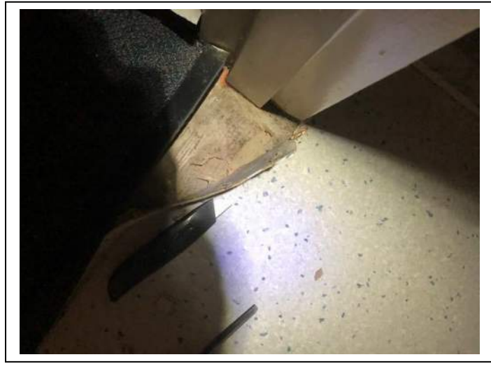
Photo #20 Material: Linoleum Sheetting With Gray Mastic Sample Result: No Asbestos Detected
