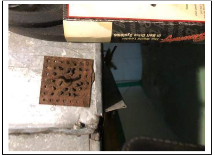
Photo #12 Material: Brown Pin Mastic Sample Result: 40% Chrysotile
