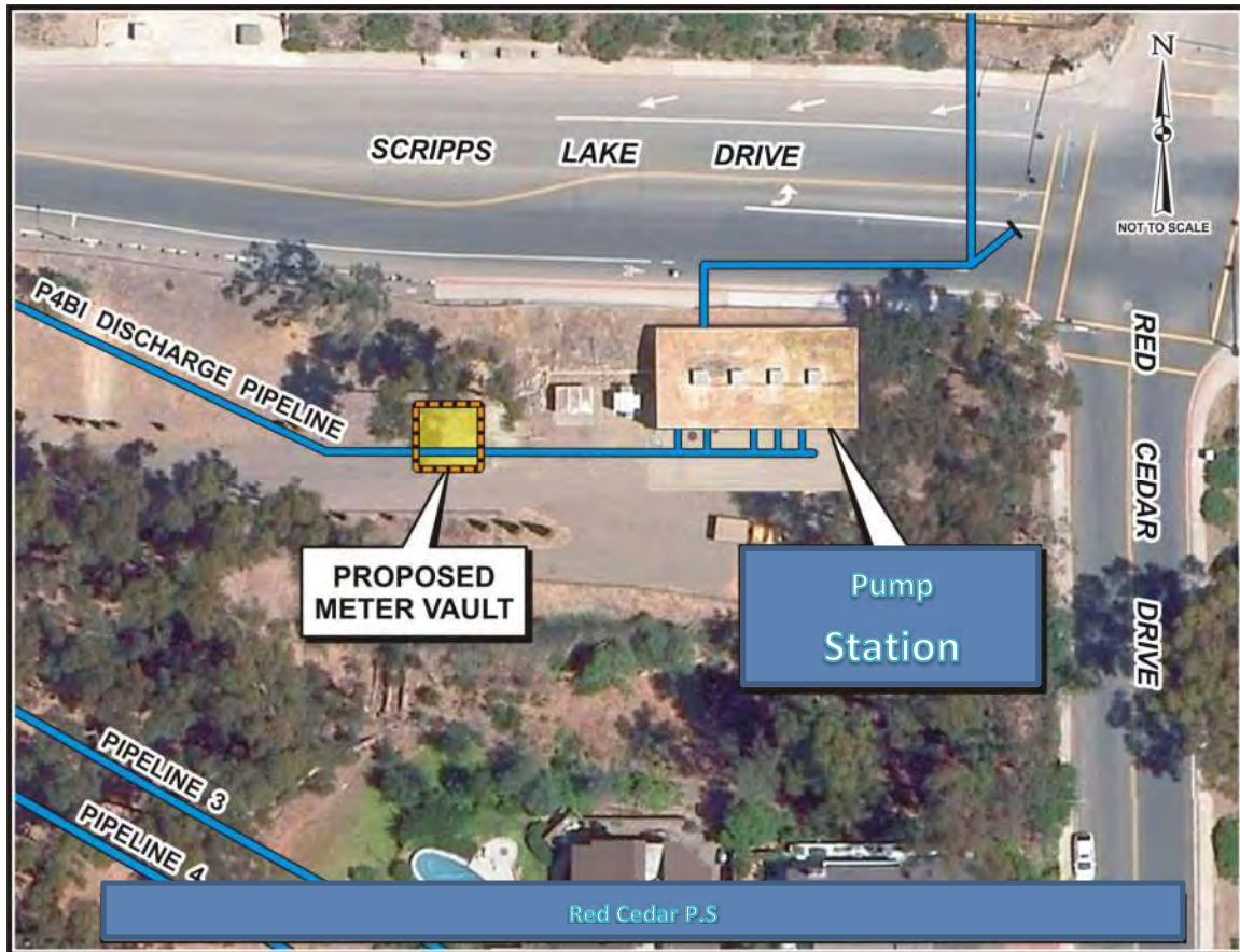
Appendix 6: Site picture with Manhole location and system flow
