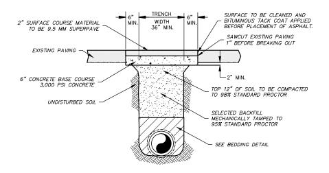
TYPICAL PAVEMENT PATCH DETAIL FOR APARTMENT COMPLEX N.T.S.
