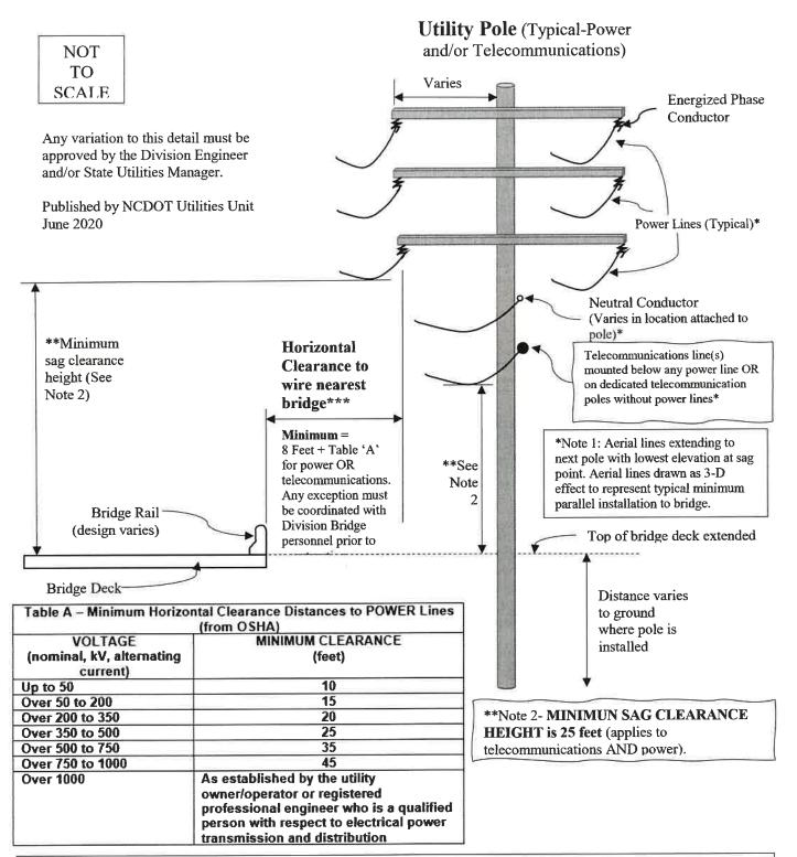
\*\*\*Note 3: HORIZONTAL CLEARANCE EXCEPTION. If vertical sag clearance height for power above bridge deck is ≥ 45 feet AND voltage is ≤ 350kV, then Minimum Horizontal Clearance may be reduced to 3 feet. Any telecommunications attachment to power pole allowed in this exception must have a minimum 25 feet sag clearance height above bridge deck.
