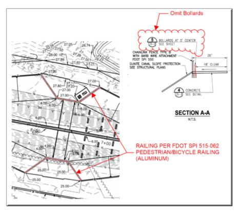
A1: Correct, delete the bollards along the top of the slope. We are still constructing fence along the top of the slope. Add safety railing where we showed it in red (this is the area of vertical drop).
