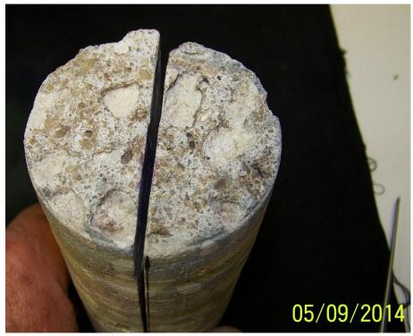
**Photo 3** – Sample 3B – end view, note surface erosion.
