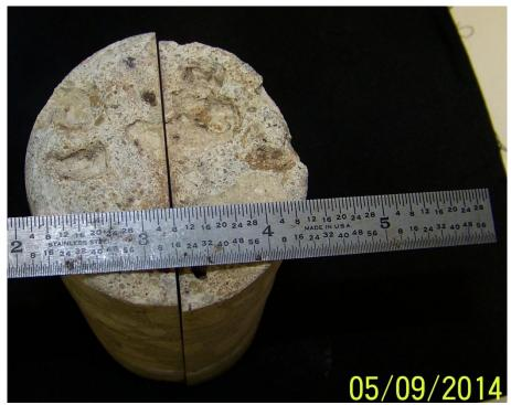
**Photo 2** – Sample 2B – end view, note surface erosion.
