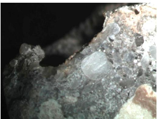
**Photo 5** – Sample 3B – magnified view of eroded surface.
