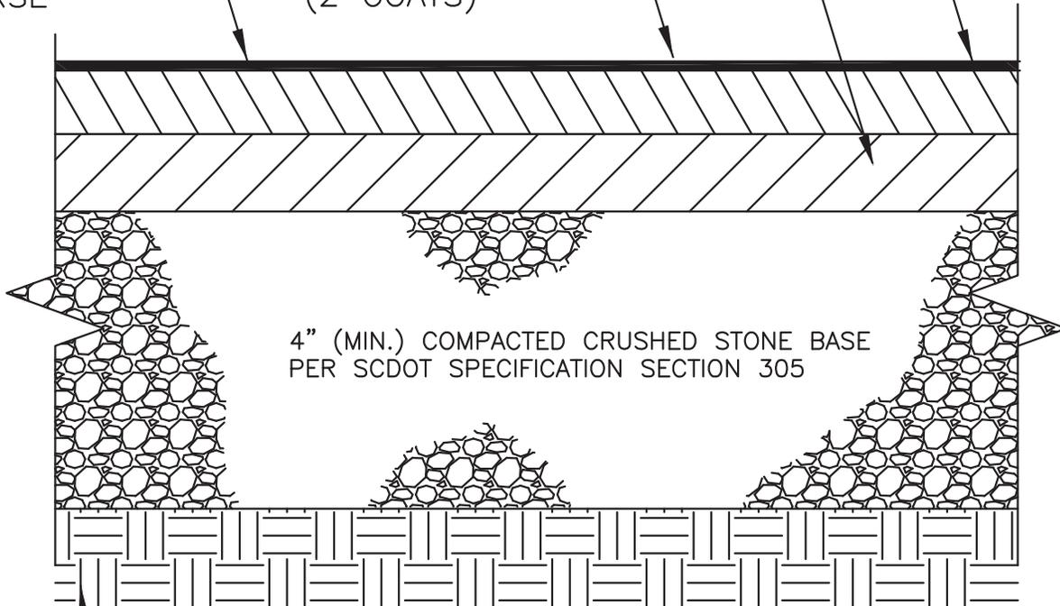
4" (MIN.) COMPACTED CRUSHED STONE BASE
