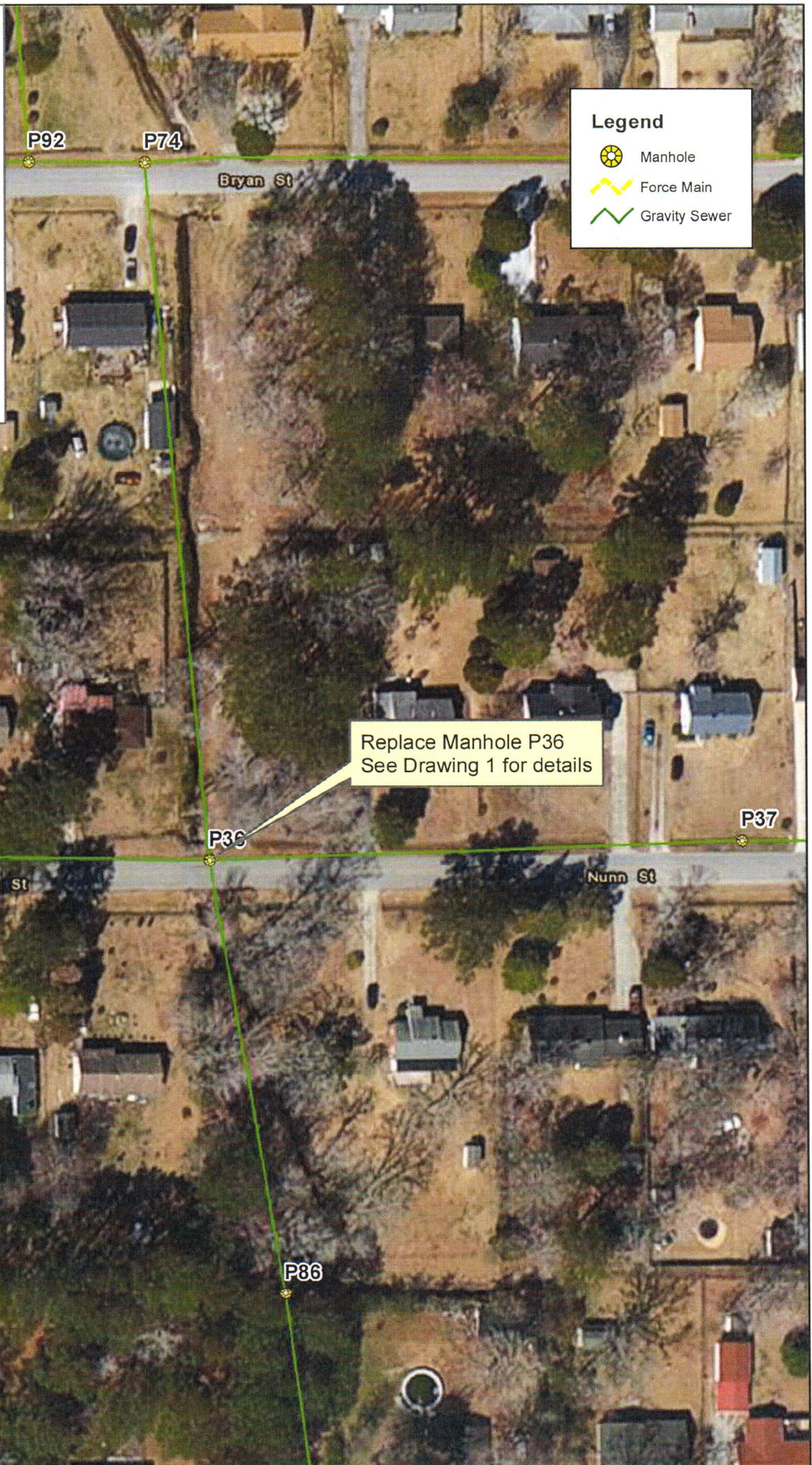
Figure 3 Manhole P36 Replacement
