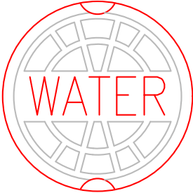
POTABLE WATER COVER
