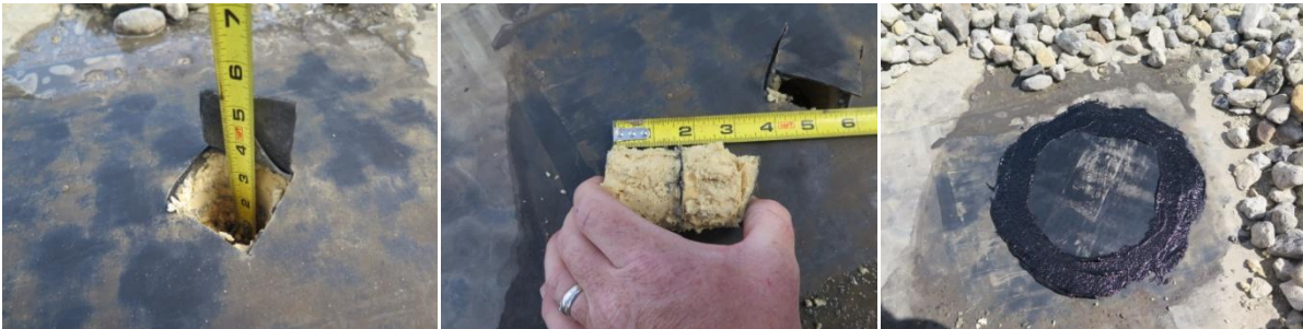
Core #2 – Metal Deck, 3" ISO, Ballasted EPDM - Dry
