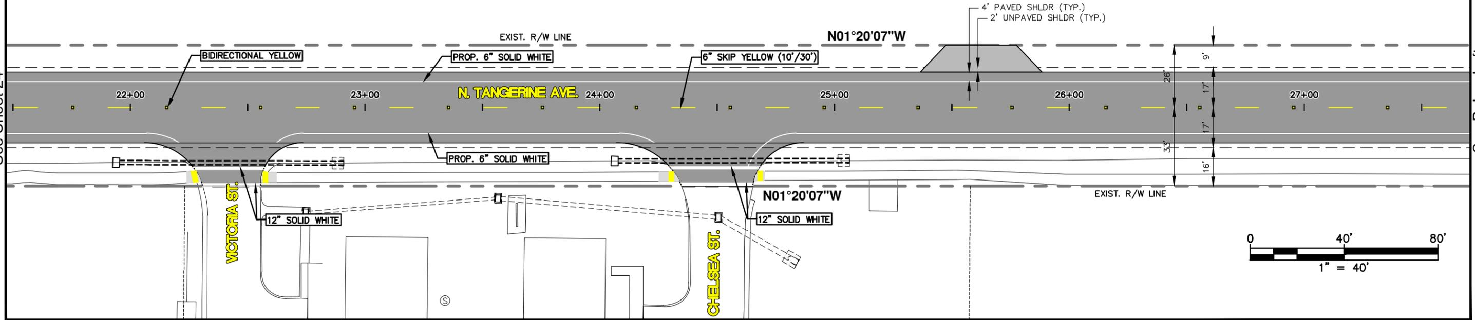
NOTE: SIGN HEIGHTS SHALL BE MINIMUM OF 7' TO A MAXIMUM OF 8' AS MEASURED FROM THE BOTTOM OF THE SIGN TO THE TOP OF THE CURB, OR IN THE ABSENSE OF CURB, MEASURED VERTICALLY FROM THE BOTTOM OF THE SIGN TO THE ELEVATION OF THE NEAR EDGE OF THE TRAVELED WAY.
