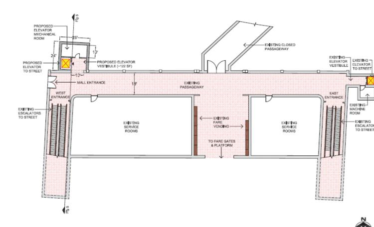
Figure 2: Existing Conditions - Passageway/Mezzanine Level
