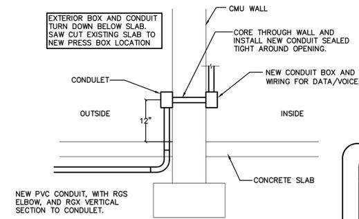
DATA & POWER THRU EXTERIOR WALL DETAIL
