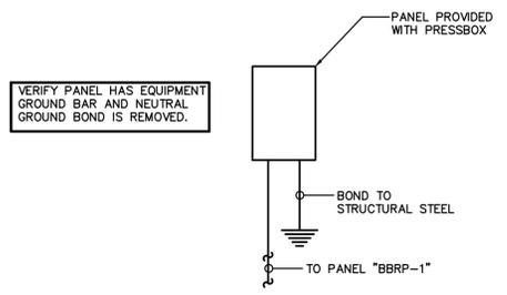
ELECTRICAL RISER DIAGRAM - PRESSBOX
