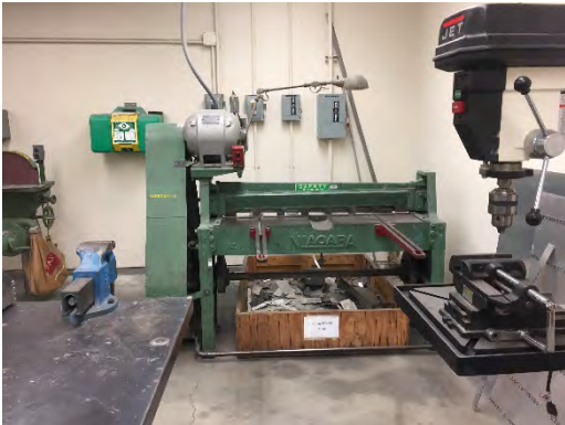
Sheet metal cutter, older, functional
