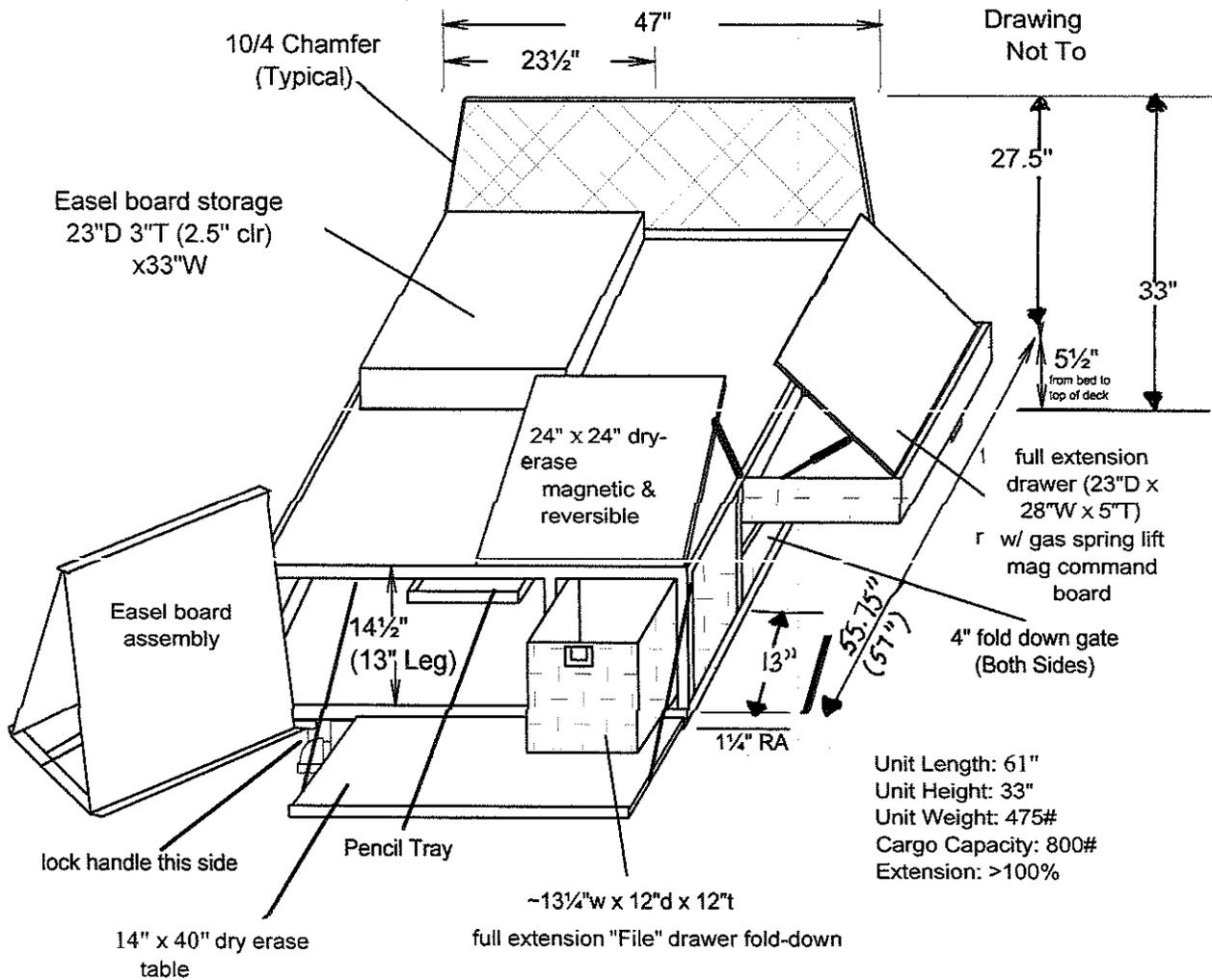
Platforms will be 0.5" birch with protective coating. Carrier will be built of 1/8" steel angle, with 1.5" 10-gauge steel mesh screen material. Fold-down table will be dry-erase polypropylene. Power lift map boards and corner easel will be of porcelain coated sheet metal, all in metal frames. Drawers will be .080 diamond plate aluminum on 300" capacity slides.
