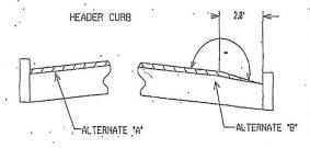
NOTE: METHOD OF FEATHERING AT PAVEMENT EDGE ALTERNATE A OR ALTERNATE B) SHALL BE DETERMINED BY THE ENGINEER. UNDER NORMAL CONDITIONS, ALTERNATE A SHALL BE USED FOR FEATHERING UNLESS RESURFACING HAS REDUCED THE "EFFECTIVE HEIGHT" OF THE EXISTING CURB TYPE FACILITY. IN THIS EYENT, ALTERNATE "B" SHALL BE USED.
