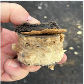
4.2 TEST CORES FROM SECONDARY ROOF
