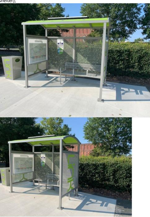
• Bus shelter, small footprint class (requires  $\leq 2$  feet of depth to install) w bench with two delineator bars, solar lighting, map case (48" x 60") (panel on roof, capable of providing light to the shelter through lights installed inside the shelter);
