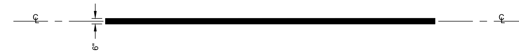
TAXIWAY CENTERLINE DETAIL NOT TO SCALE
