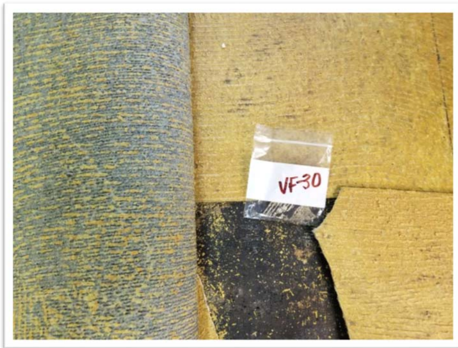
Photograph #06 Sampling Point VF-30, Below Carpet in Hall – 12”X12” VFT/Mastic (4% Chrysotile / 6% Chrysotile).
