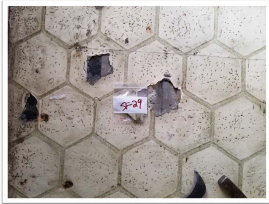
Photograph #05 Sampling Point SF-29 in Galley – Cream w/ Green Trim Hexagon Vinyl Sheet Flooring (15% Chrysotile).
