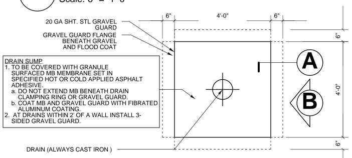
**Drain Gravel Guard Detail Plan**Scale: 1/2" = 1'-0"
