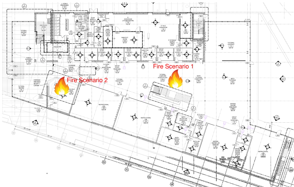
Figure 2– Fire Locations on Level 1
