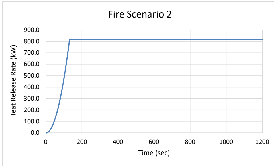
Figure 5– Scenario 2 Reception Area Fire Curve
