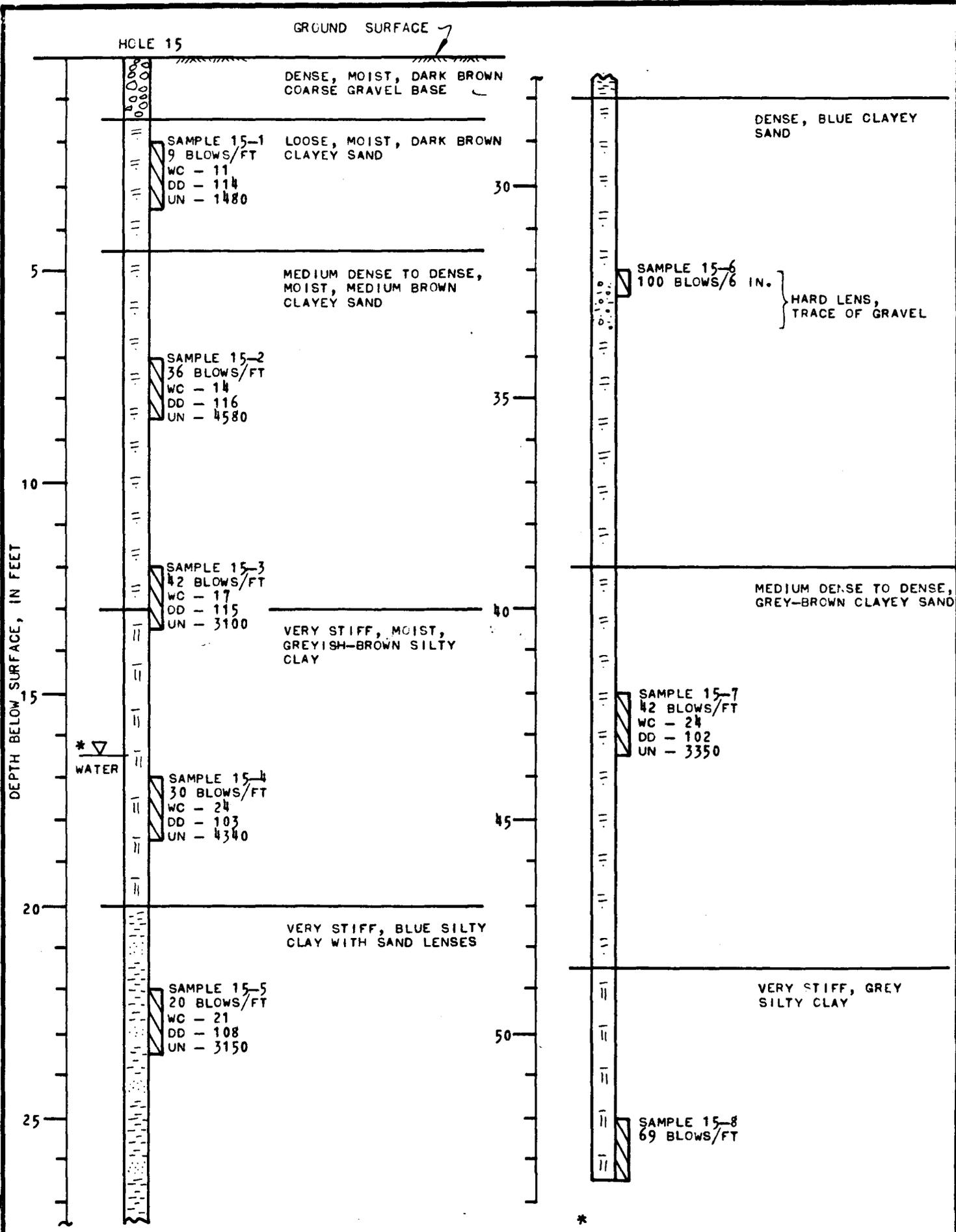
FIG. 23 - LOGS OF BORINGS
